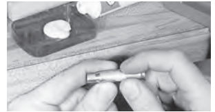
Carbide dies need no lubrication
