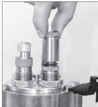
Thread assembly into powder through expanding die or rifle charging die
