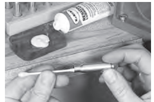
RIFLE DIES ONLY Be sure to lube inside of the case neck with a cotton swab.
