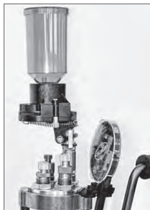
Thread assembly into powder through expanding die or rifle charging die
